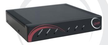
UHP-100 is equipped with two high-speed demodulators together with their independent IF inputs and front ends. The router can simultaneously receive two carriers transmitted via two different satellite beams, which can even be in different frequency bands. The dual demodulator in conjunction with a built-in advanced beam switching algorithm facilitates seamless roaming of mobile satellite terminals between distinct beams of HTS satellites.
